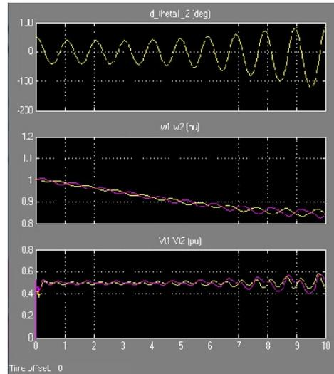
Fig. 7.  $d_{\theta}$  angle of without STATCOM.
