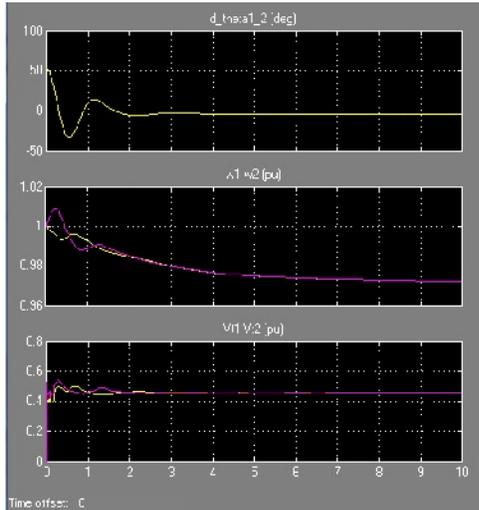
Fig. 8.  $d_{\theta}$  angle of with STATCOM.
