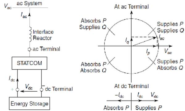
**Fig. 4.** The power exchange between the STATCOM and the ac system.
