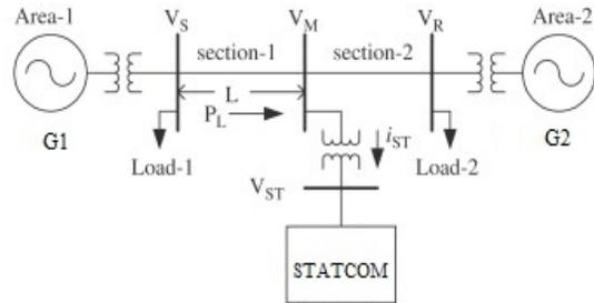
**Fig. 5.** Single line diagram infinite bus with fault.
