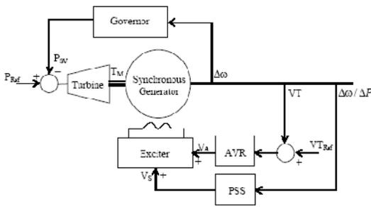
Fig. 1. Generation unit diagram.
